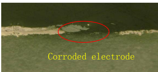
Figure 1 Left top terminal is corroded
